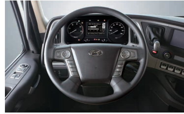
Steering wheel (Including pneumatic tilt and telescopic function)
