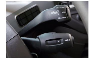
Multifunction automatic shift lever (AMT) The automatic shift lever makes it easier to change gears in the driver's cab.
