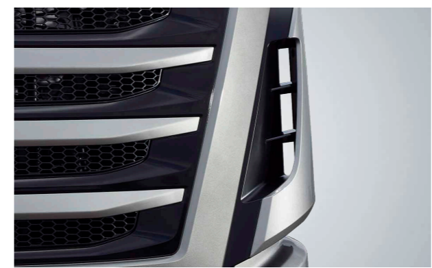
Application of bumper vane to reduce side contamination
