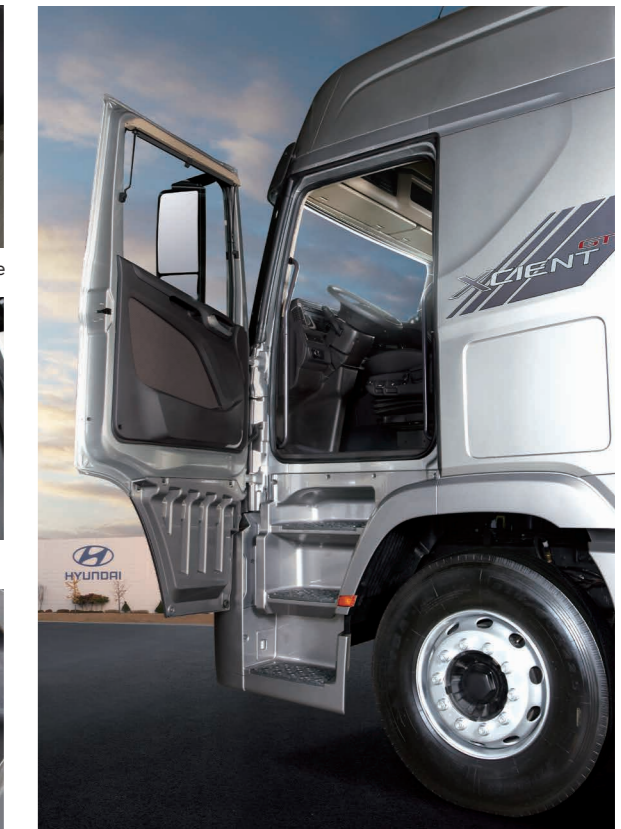
Inclined steps with the largest cross-sectional area in its class
